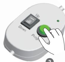
Press the Program button in the DC270(A/I), the motors will rotate in a clockwise direction, Release the Program button namely confirm clockwise limit position
