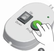
Press the Program button in the DC270(A/I), the motors will rotate in a Counter-clockwise direction, Release the Program button namely confirm Counter-clockwise limit position
