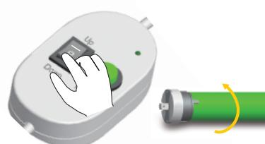
Press the DOWN button in the DC270(A/I), the motors will rotate in a Counter-clockwise direction or stop
