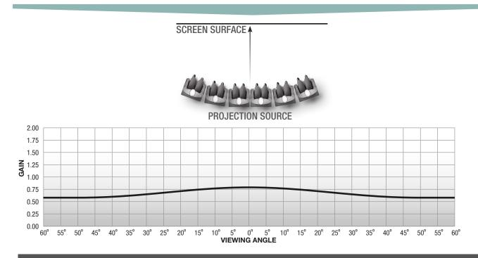
GAIN 0.8 VIEWING ANGLE 180° THICKNESS 0.3 MM 8K COMPLIANT
